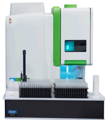
4DXCi SampleSense Oil Analysis System with Avio 500 ICP
